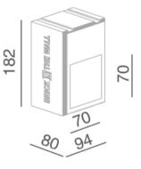
Ready for installation in solid walls Optional plasterkit for installation into gypsum walls
